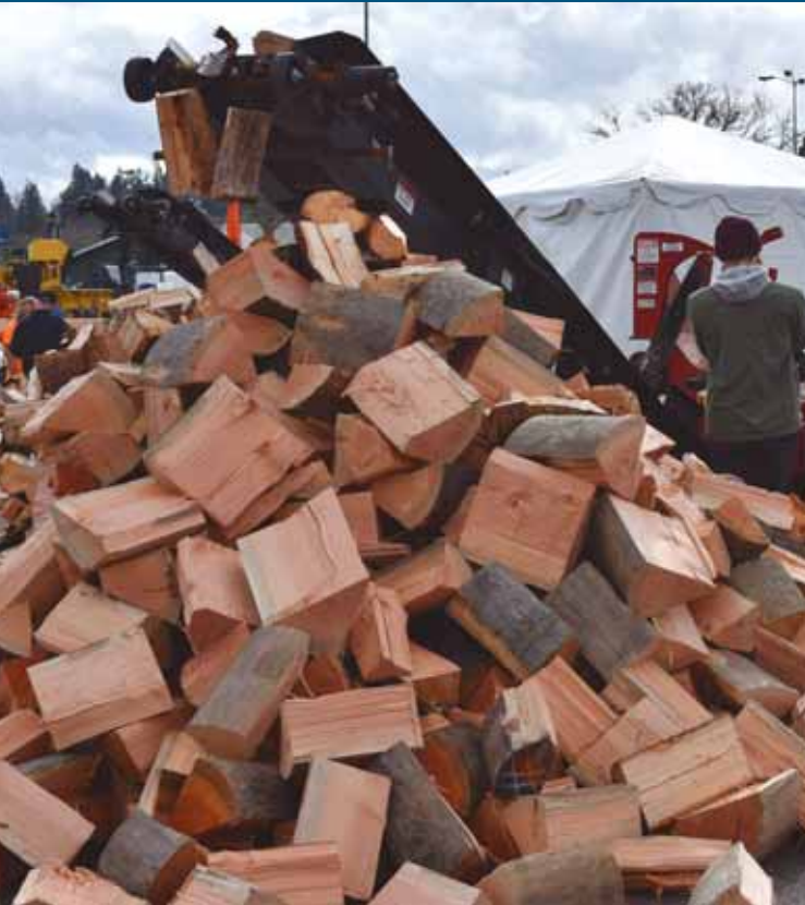
The hydraulic conveyer on the outfeed swivels 3 feet to spread the firewood across a broader area.
