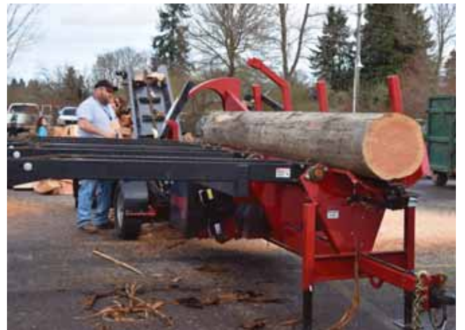
The standard hydraulic log deck features three strands. Jim modified his deck, placing strands in 15.5-inch increments, and also extended the deck to 16 feet so that he can handle logs from 3 to 26 feet.
